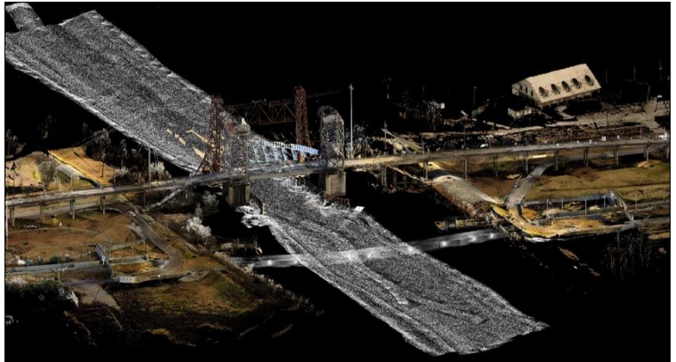
Laser Scan and Hydrographic Survey of Belle Chasse Bridge and Tunnel project area
