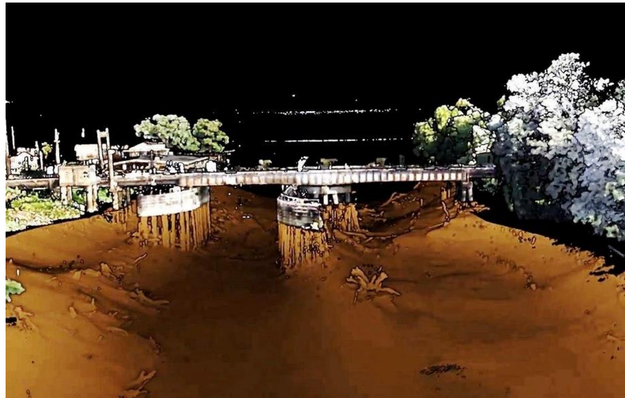
Port Vincent Bridge Scan and Bathymetry Integrated
