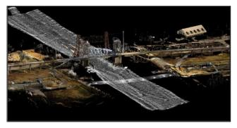
Forte and Tablada provided comprehensive topographic surveying services for the Belle Chase Bridge and Tunnel Replacement project for LA DOTD. Included in this work was a survey performed utilizing traditional methods, terrestrial laser scanning of roadway surfaces, and multi-beam 3-D hydrographic surveying.
