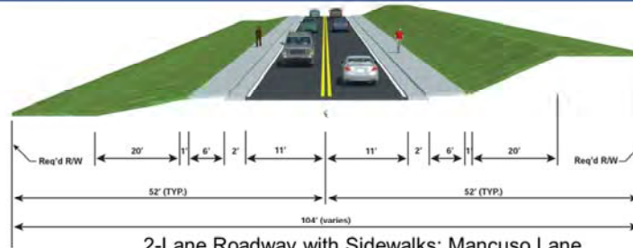
2-Lane Roadway with Sidewalks; Mancuso Lane
