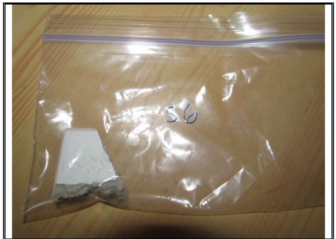
Photograph No. 017: Sample 6 – Drop ceiling tile
