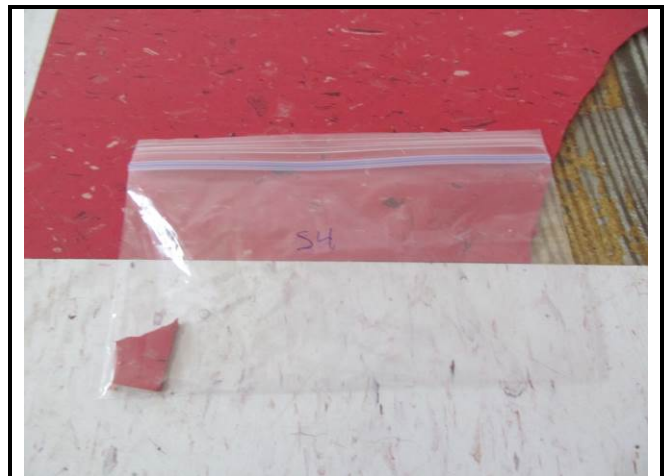
Photograph No. 012: Sample 4 – Red vinyl floor tile 12x12
