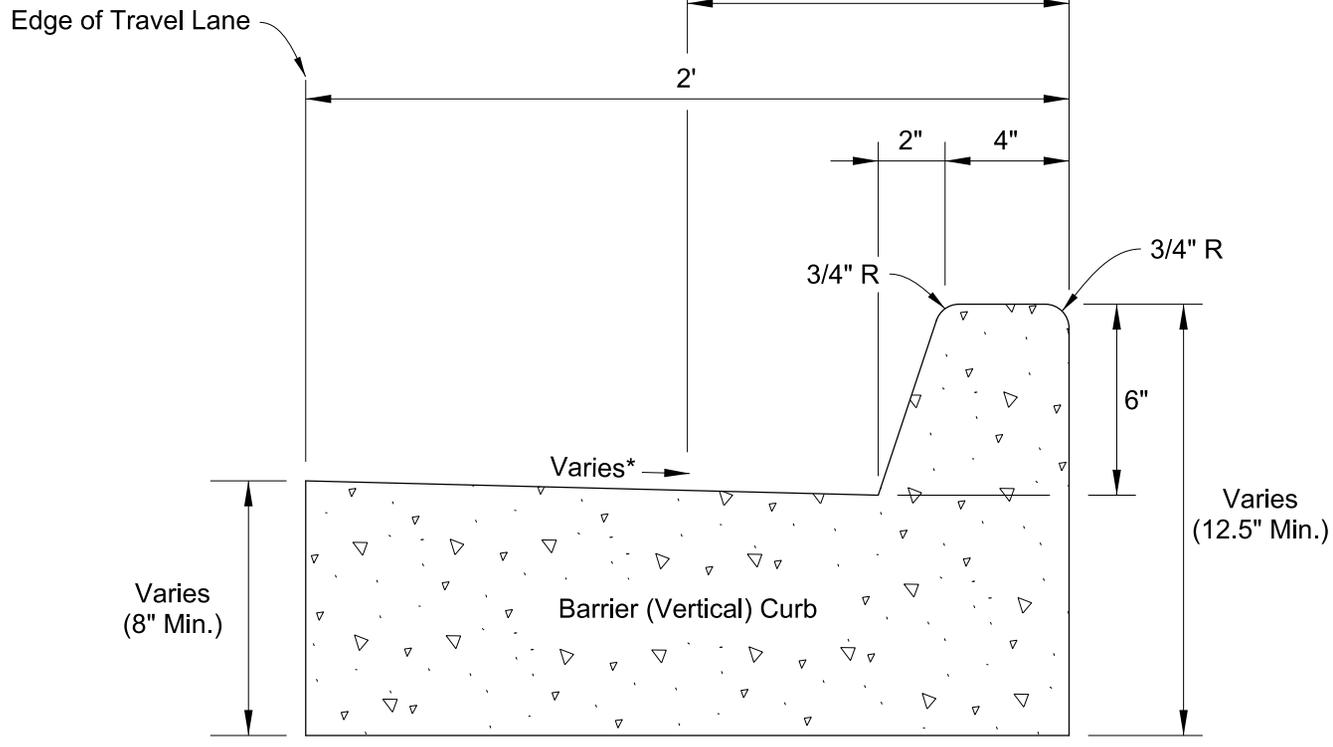
\*The gutter slope will typically match the cross slope of the roadway (normal crown or superelevation).
