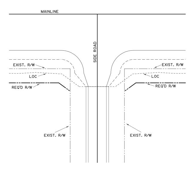
FIGURE 8-21: LIMITS OF CONSTRUCTION IN PLAN VIEW
