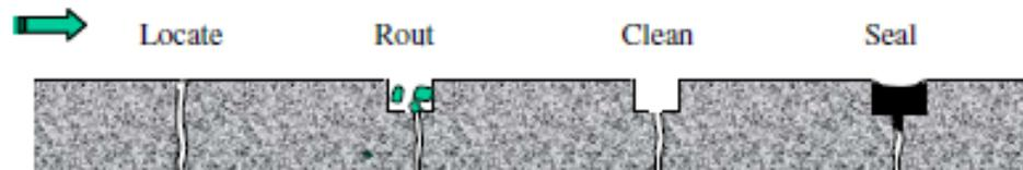
Illustration of Crack Routing, Cleaning, and Sealing
