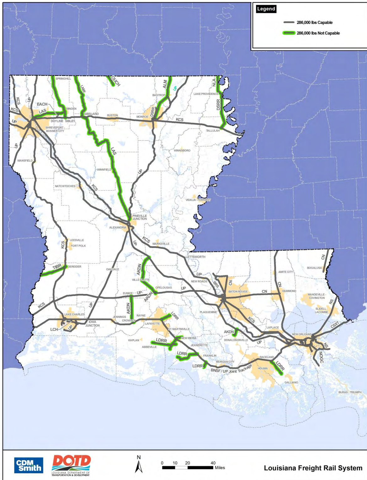
Figure 2-2: Lines Incapable of Handling Car Weights of 286,000 pounds
